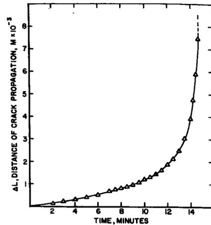
Fig. 2. Crack propagation to failure under constant load, tested in air at 50% rh.
