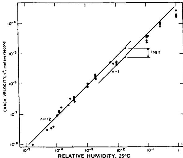
Fig. 6. Dependence of crack velocity  $v^+$  on water vapor concentration in the environment. Data were taken from region II. Lines labeled  $n = 1/2$  and  $n = 1$  represent the theoretically predicted behavior at low and high concentrations of water vapor, respectively.
