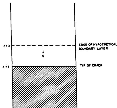
Fig. 4. Cross section of a microscope slide showing crack surface. The cross-hatched area indicates the unbroken portion of the slide.
