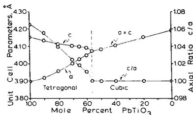
Fig. 4. Unit cell parameters and axial ratios as a function of mole percent  $\text{PbTiO}_3$  in  $\text{BaZrO}_3$ .
