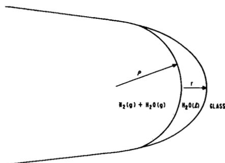
Fig. 7. Schematic diagram of a water pocket at a crack tip.
