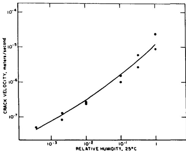
Fig. 5. Dependence of the crack velocity on water vapor concentration in the environment. Data were taken from region I with constant applied force of 0.8 kg. The curve represents the formula  $v = 2.11 \times 10^{-6} y^{1/2} + 1.02 \times 10^{-4} y$ , where  $y$  is relative humidity.
